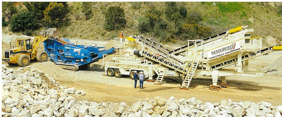
Mobile Crushing Circuit - 42-30 Pegsun Crusher feeding an Alliss Chalmers 45 cone crusher feeding into a 16 x 16 Hawk screen capable of producing 250 tonnes per hour of a full range of quarry products.
